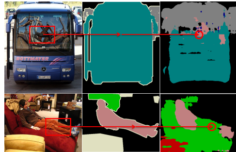
Figure 1. Illustration of the misclassification examples. Images in the left column are the original images, the center column shows the ground truth, and the right column shows the prediction result of the baseline model.
